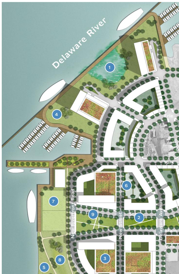
1. Constructed wetlands store and filter excess stormwater, permit infiltration, and enhance biodiversity.
