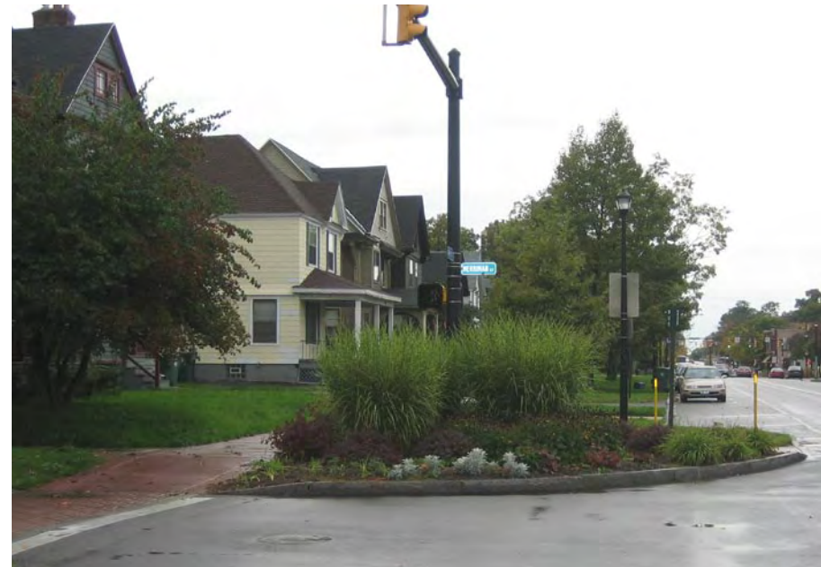
Bump-out to help pedestrians cross 2nd Street in Northern Liberties, Philadelphia, top. Planted bump-out and brick-paved crosswalk in Rochester, NY.
