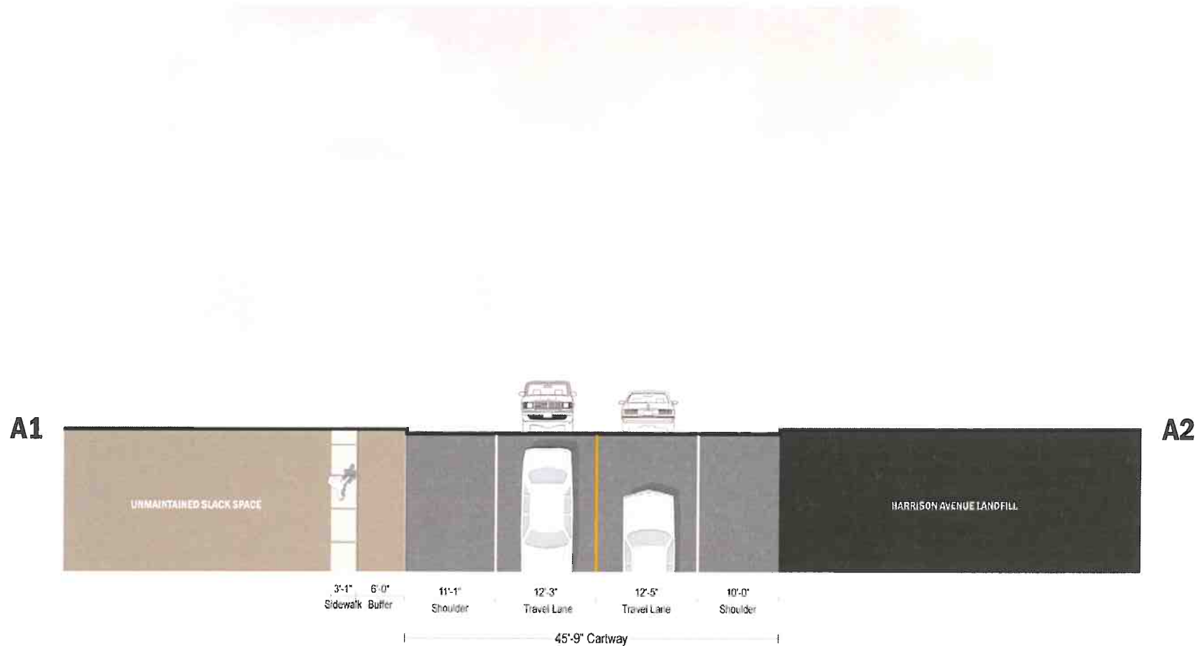
Figure 58. Existing State Street between Centennial Drive outlet and State Street Bridge
