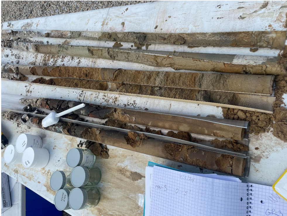
September 5, 2024 – Soil boring GP-4. Macrocore core liners 0-5 feet, 5-10 feet, 10-15 feet shown.
