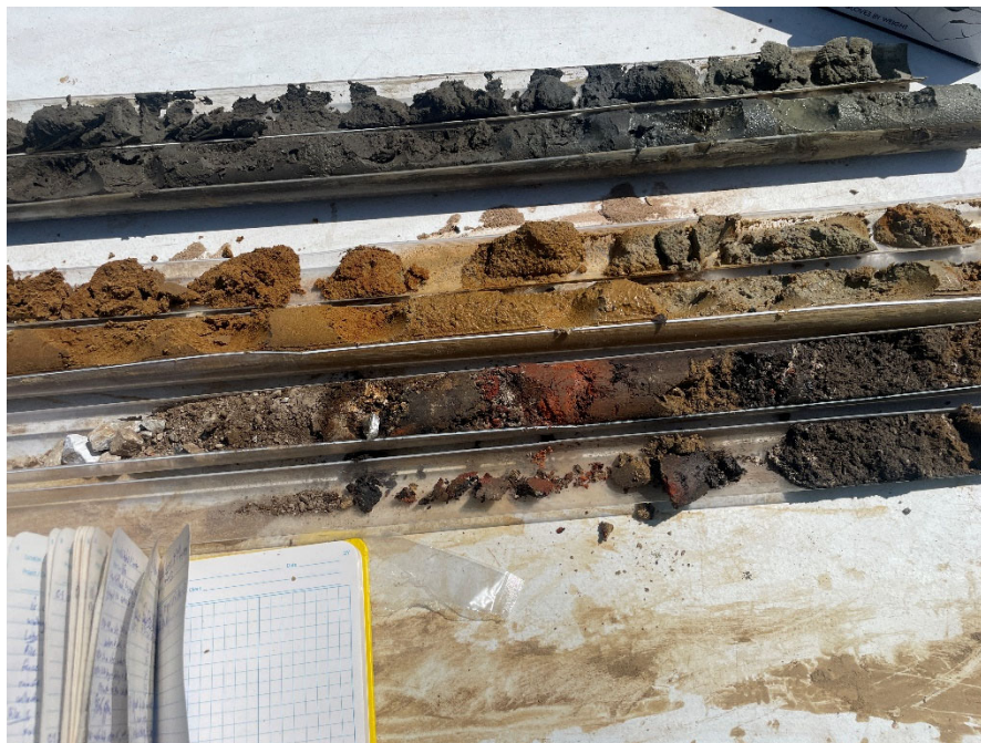
September 5, 2024 – Soil boring GP-2 (MW-2). Macrocore core liners 0-5 feet, 5-10 feet, 10-15 feet shown.
