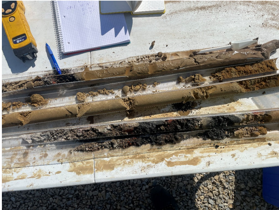
September 5, 2024 – Soil boring GP-1. Macrocore core liners 0-5 feet, 5-10 feet, 10-15 feet shown.
