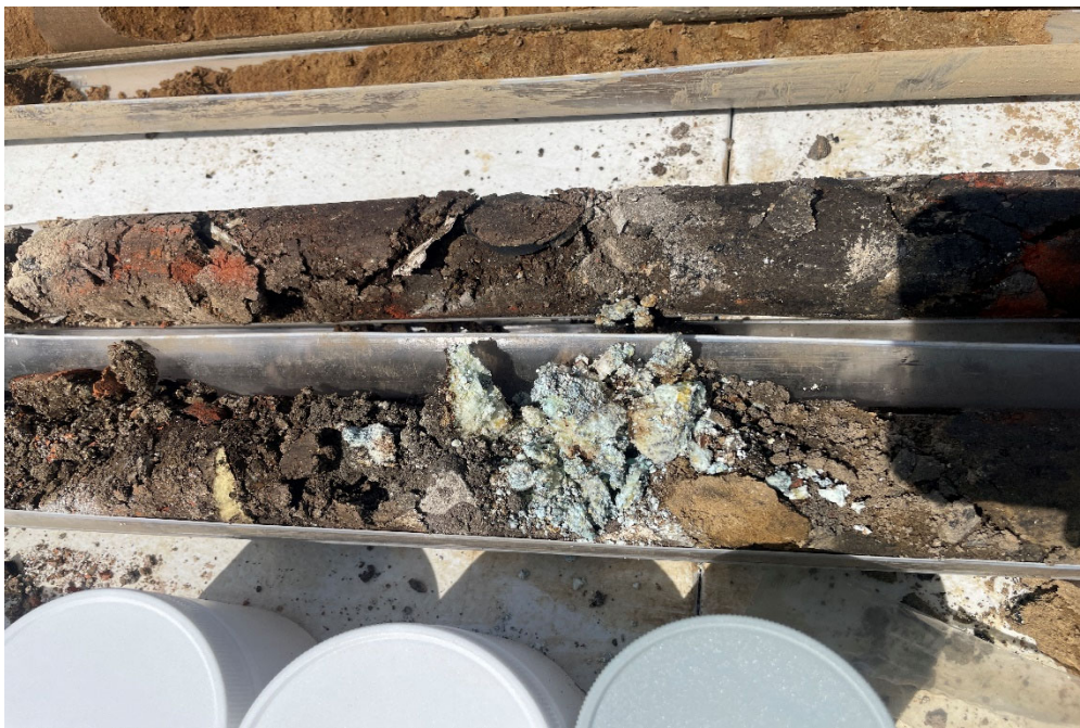
September 5, 2024 – Soil boring GP-4. Staining observed at 1-1.5 feet bgs.
