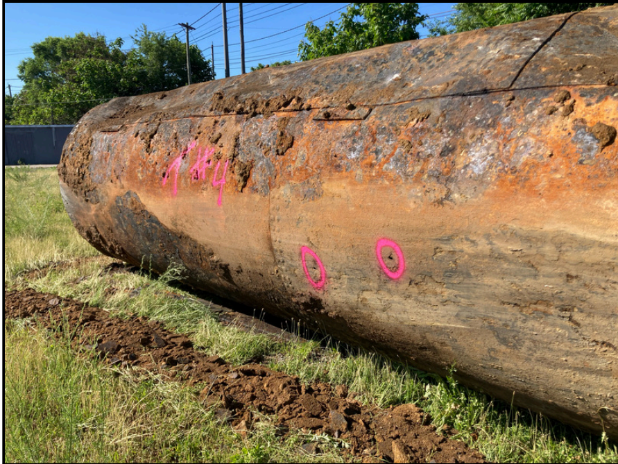
Holes circled in pink on the bottom of AOC 1E
