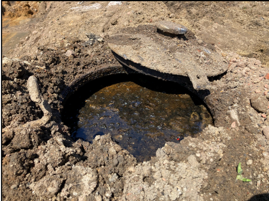
Residual product and water mixture within AOC 1B
